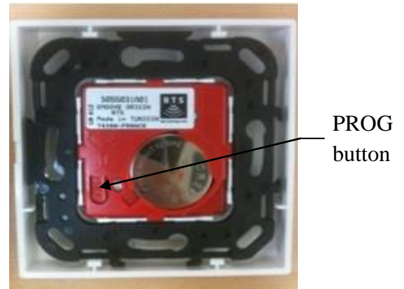
Back of Wall Switch
